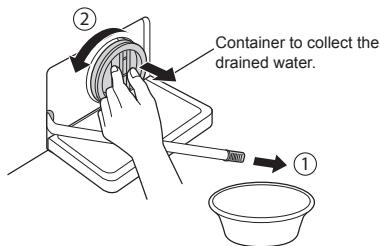
3 Remove any extraneous matter from the pump filter.
